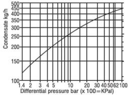
Note: Minimum Differential pressure for satisfactory operation 1.4bar g with Positive Pressure and Discharge to atmosphere.
